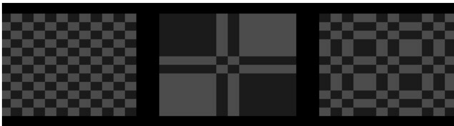
Figure 9-4 GL_REPEAT, GL_CLAMP_TO_EDGE, and GL_MIRRORED_REPEAT Modes
