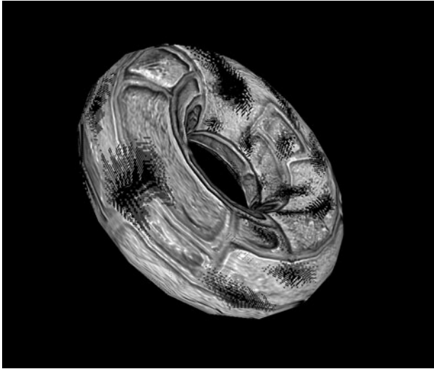
Figure 5-3 Z Fighting Artifacts Due to Not Using Invariance
