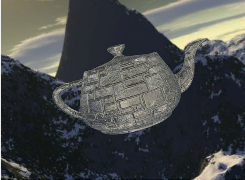
Color Plate 5 (see also Figure 13-2) Environment Mapping example. This example uses a cubemap to perform environment mapping. The eye-space reflection vector is computed in the fragment shader based on the normal vector stored in the normal map.
